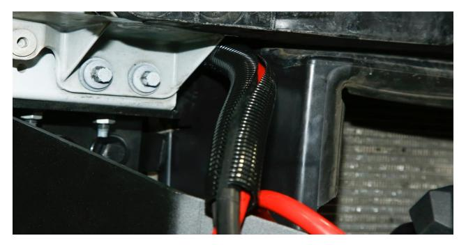
Position the solenoid in the side of the winch tray, make sure the wiring is sitting neatly then fit and tighten the supplied M8 bracket bolts. Secure the wiring with cable ties, then remove the paint and attach the solenoid earth to the stud on the back of the square section.
