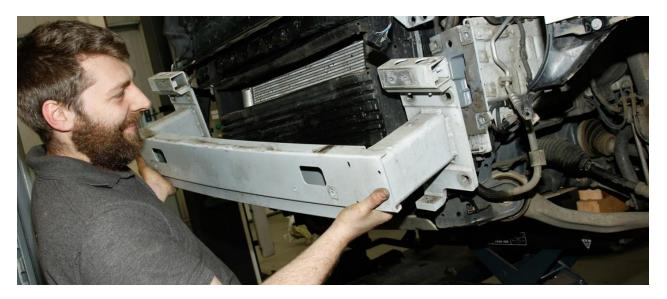
The plastic guard that runs behind where the crash bar was needs to be trimmed away. Carefully slice down the sides of the radiator duct, then remove the centre. Mask off the edges of the duct, mark out the measurements in the kit instructions and trim away.
