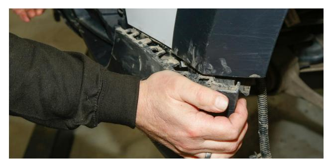
Refit the headlamp surrounds and plumb the washer nozzles, then clip the foglamp surrounds back in. Fit the upper grille, then finally the slam panel cover, being sure to use the correct fixings in the right places. Leave the metal bash plate off for now.
