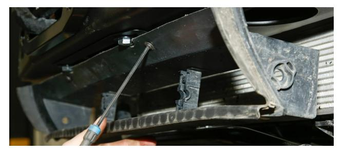
Use a saw to cut through the upper piece of ducting, removing the supports and lower horizontal piece. Cut up to the edge of the lower corners, as shown, so that the duct corners sit neatly on the winch tray when in place. Test fit and trim as needed.
