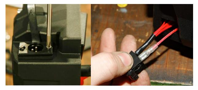
Cut the red multiple wire connection with black connector to the on off switch and join the extension loom yellow wire with blue crimp connector to the red multiple wires. Connect the red spade connector on the other end of the yellow wire to 'O' side of the on off switch.
