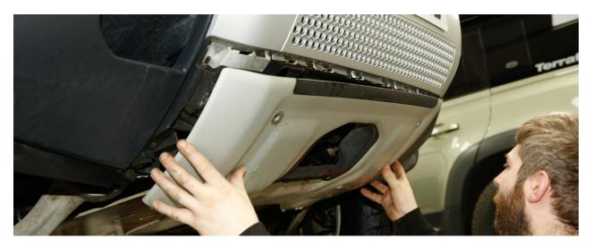
With the front wheels off, release the four plastic pin clips and four screws that secure each inner arch liner, then remove them. Release the tabs and remove the plastic brake ducts – once out of the way, undo the 10mm wing bolts and unclip the ends of the bumper.
