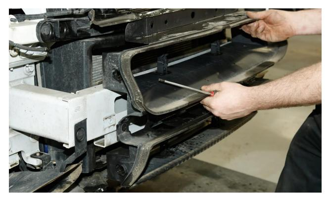
Loosen and remove the four 15mm bolts that hold the tubular lower crash bar in place and remove it. This will be refitted once the Terrafirma winch tray is in place and will be held to the bottom of the winch mount with dedicated brackets.
