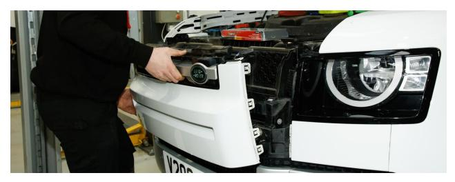
Use the trim tool again to access and press down the clips around the outside of each foglamp surround and lift them away. Now jack up the front of the vehicle, secure it on stands and remove the front wheels to gain access to the back of the bumper.
