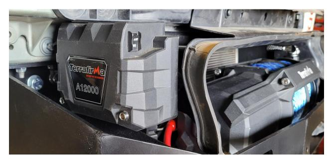
Route the black earth and red power cables around the inside of the inner wing and up to the rear left corner of the engine bay. Undo the nut on the earth jumper post, fit the earth cable beneath it, then spin the nut back on and nip it up.
