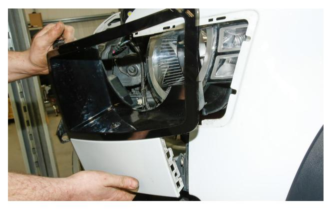
Undo the 10mm screws along the top and T30 screws along the base, then lift the bumper off. Let it rest on its back or sit it forward on a soft towel or sheet to prevent scratches. Attend to the silver bumper section later.
