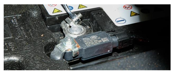
Disconnect the battery. Access it by moving the driver's seat forward and lifting the hatch below, then loosen and remove the earth cable. Land Rover may call and confirm your vehicle isn't being stolen.
