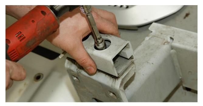
With assistance, lift the winch tray up and into place and push the top bolts through, allowing the tray to hang. Position the nut plates behind and start the new bolts by hand; nip them up just enough to hold the tray flush to the chassis, but still allow movement.
