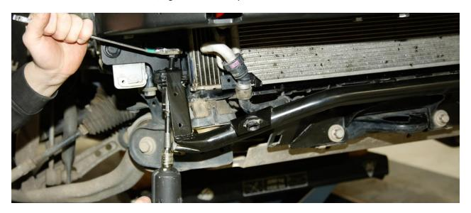
Use a sharp knife or saw to cut the two half-moon pieces off the main bumper plastic, then turn your attention to the air ducting. Cut out the paper template and tape it to the duct, making sure it's central. The duct will be cut into two pieces to clear the tray.
