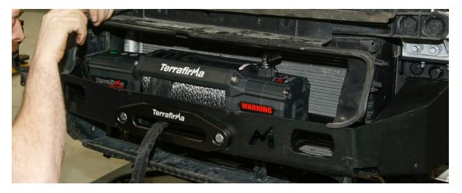
The front of the winch tray has two holes, which the centre parking distance control (PDC) sensors recess into. Route the wiring harness and position the two plugs so they poke through the holes in the tray; this will make refitting the bumper easier.
