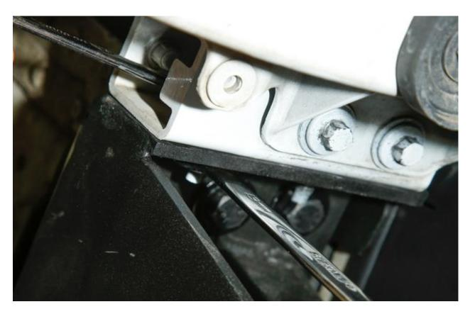
When fitting a Terrafirma A12000, the kit comes with a dedicated relocation bracket for the solenoid pack. Remove the metal backplate and swap the original mounting bracket for the one in the new kit. The space for the solenoid pack is tight, take care to use the most suitable bolt locations to position the solenoid pack correctly.
