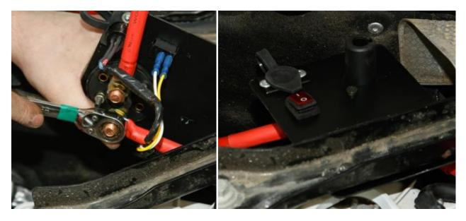
The Defender L663 has convenient pre-wired power posts in the engine bay. Unclip the cover and fit the winch power cable that runs to the isolator switch to one of the posts, along with a 500A mega fuse, and secure both with M8 flange nuts. Refit the cover.
