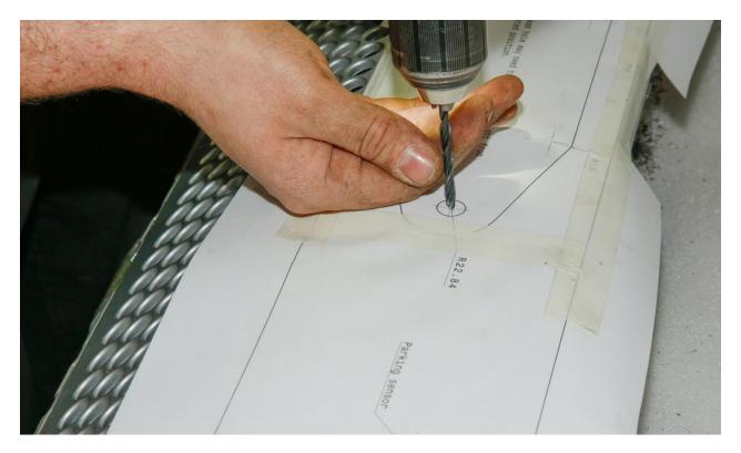
Make a cross or dot in the middle of each of the fairlead bolt heads with a marker pen or blob of paint. This will help assure that the fairlead cut-out template is perfectly positioned before you commit to making the full cut on the silver bumper finisher.
