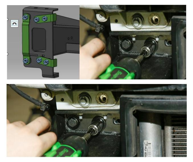
With the main winch tray and original box section pieces tight on the chassis rails, use a spanner to reach down the box sections and fully tighten them down onto the tray, holding the new M8 flange nuts on the inside of the winch tray aperture.
