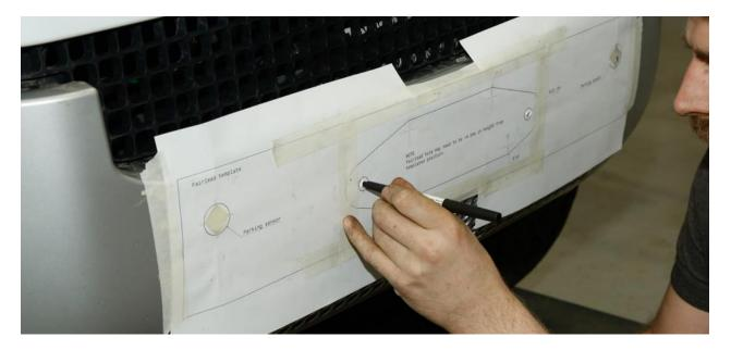
Use hole saws to cut the corners of the fairlead aperture, then carefully join the holes together with a sharp knife. File the edges smooth and check the fit of the panel, adjusting if needed. When happy, clip the panel on and secure, then refit the bash plate.
